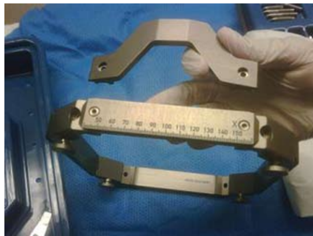
FIG. 1. Photograph of the base of the Leksell frame with the straight face plate attached and the angled face plate held in the correct position.
